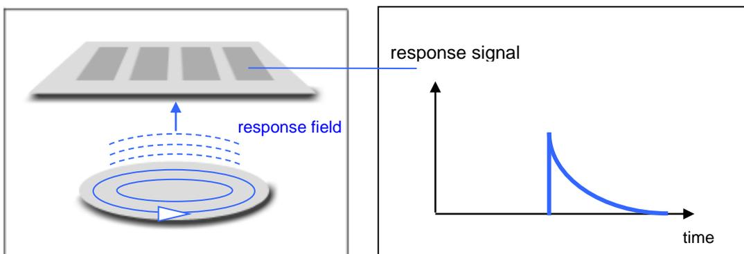
The emission field is generated by alternately switching the current on and off in very short intervals (in the range of a few microseconds). Once the emission field has completely subsided the response field is measured. In this way an overlap of the response signal and the comparatively strong emission
