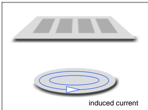
At the bottom of the layer is located a reflector (a foil or circular plate of metal). The pulsating magnetic field induces eddy currents in the reflector which subside exponentially and in turn generate a time-dependent magnetic field: the so-called response field.
