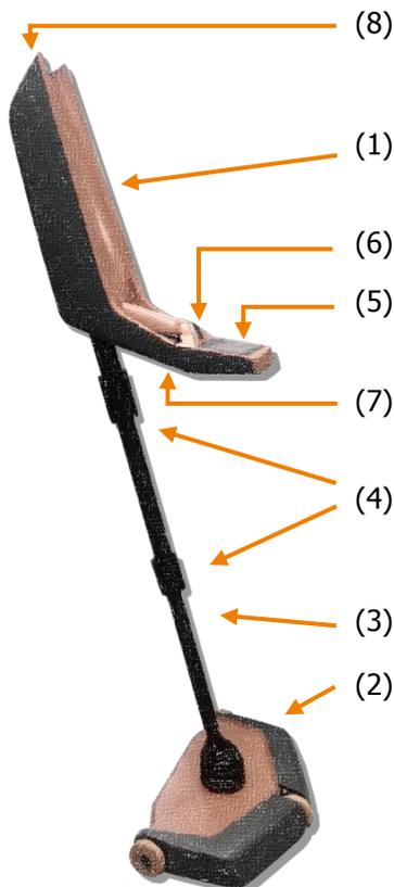
Measurement data are collected by a defined pass over the reflector. During one run, while the reflector is passed over, up to 150 position-dependent measurement points are collected by each of the four receiving sensors.
