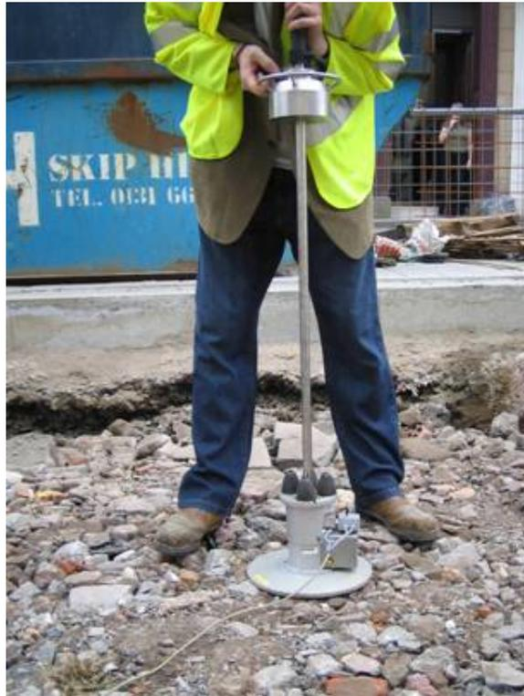
Figure 8 Testing on Large Particle Size Materials
