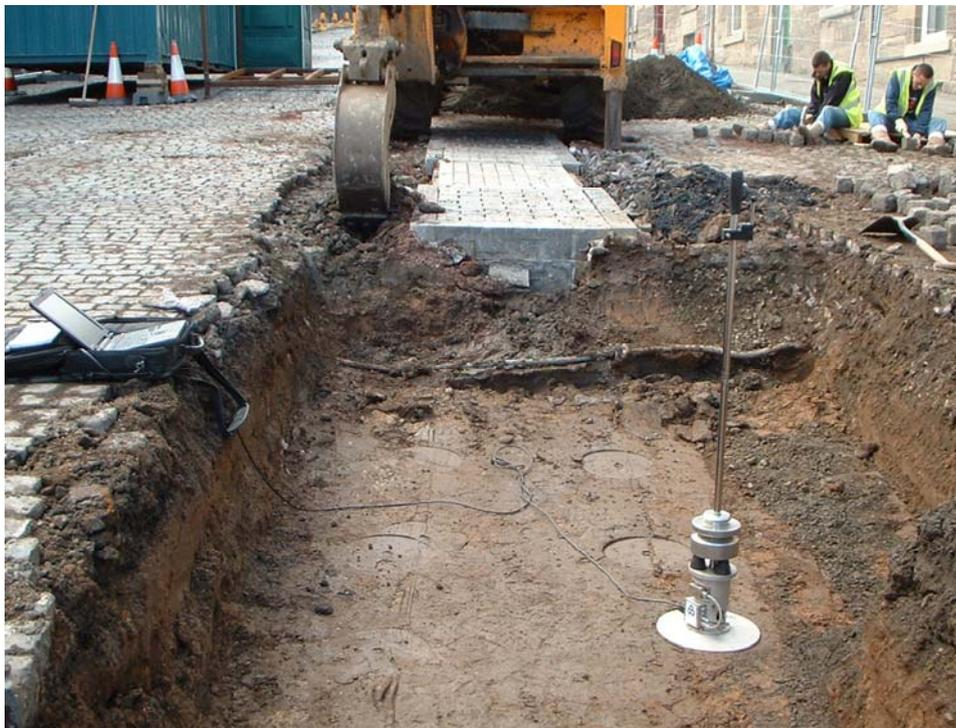
Figure 9 Shearing of Ground During Testing
