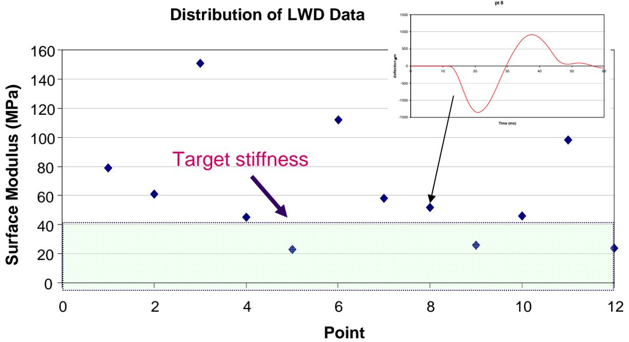
Figure 10 Sample Test Data (Note Failures at areas 5, 9 and 12, and although Point 8 is above the target stiffness examination of the signal response shows large rebound and therefore has failed)
