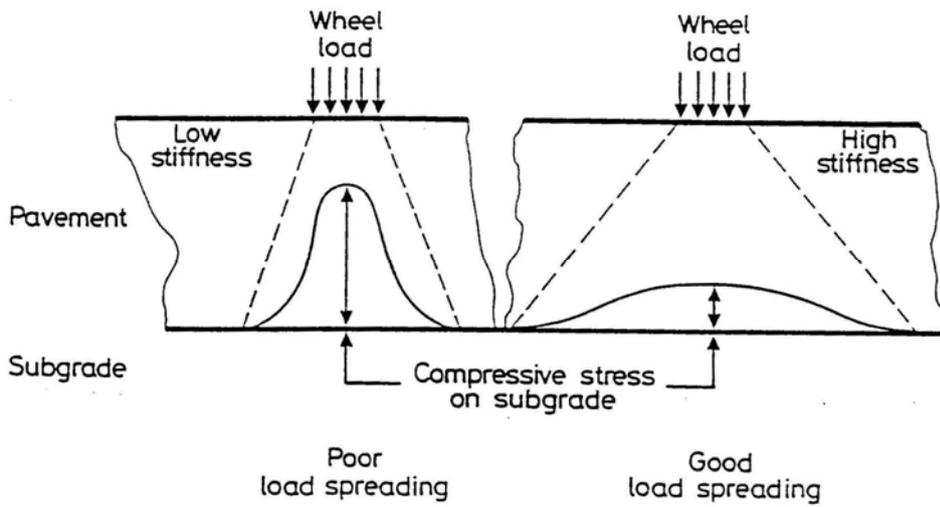
Figure 1, Pavement Load Dissipation and the Importance of Stiffness
