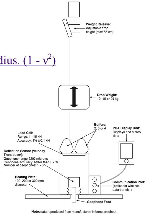
Figure 4 Schematic of and LWD Device, and the Bousinnesque Equation
